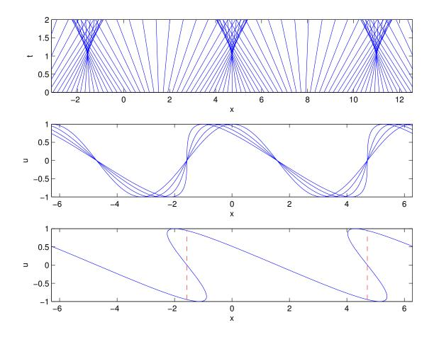
which first diverges for  $x_0 = x = -\frac{1}{2}\pi = \frac{3}{2}\pi = \frac{7}{2}\pi = \dots$  at t = 1. (3 points). The integral form of the conservation law is
